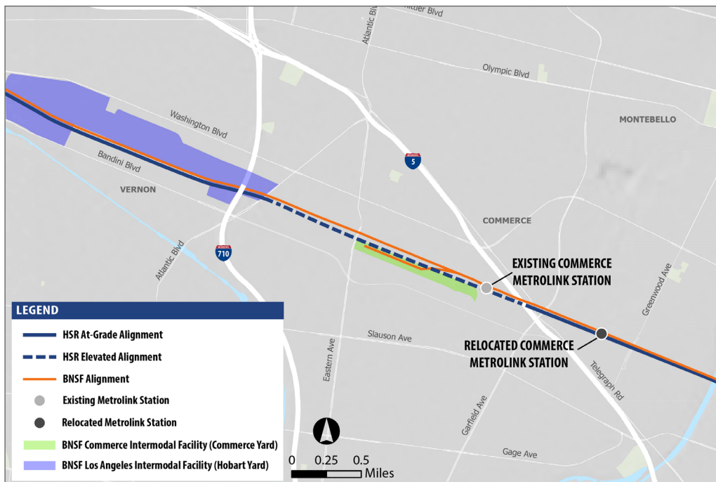
Commerce Metrolink Station Relocation
