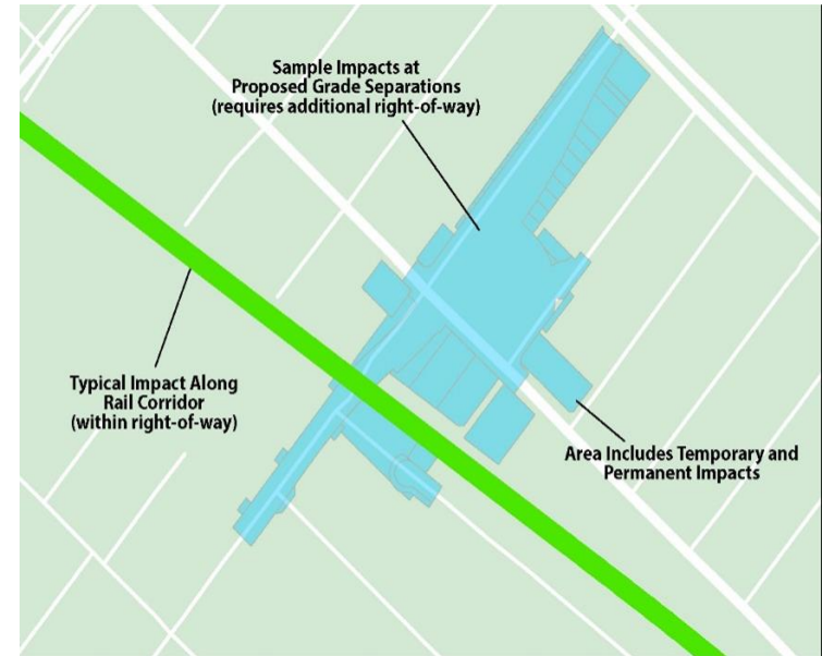
Sample Impacts at Grade Separation
